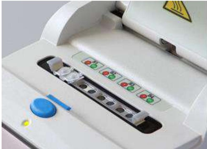
***The reaction strips must be loaded IN THE CORRECT ORIENTATION as shown above, with hinges towards the rear of the instrument.***
