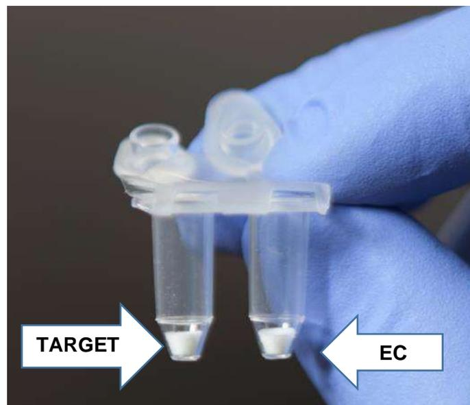
4. Peel off the plastic seal on the tubes carefully, taking care not to disrupt the lyophilised pellet. (If lyophilized pellets are sticking to the sealing film, tap the strip lightly until they fall to the bottom of the tubes.)
