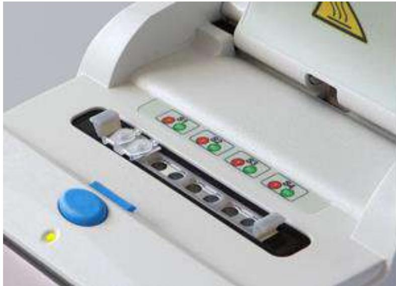
***The reaction strips must be loaded IN THE CORRECT ORIENTATION as shown above, with hinges towards the rear of the instrument.***
